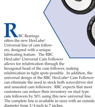
The RBC HexLube® Universal Cam Follower design provides the easiest and fastest way to relubricate cam followers in hard to reach places or in applications where stud access is limited. A cam follower that is properly maintained and lubricated will last longer than a cam follower that is neglected
