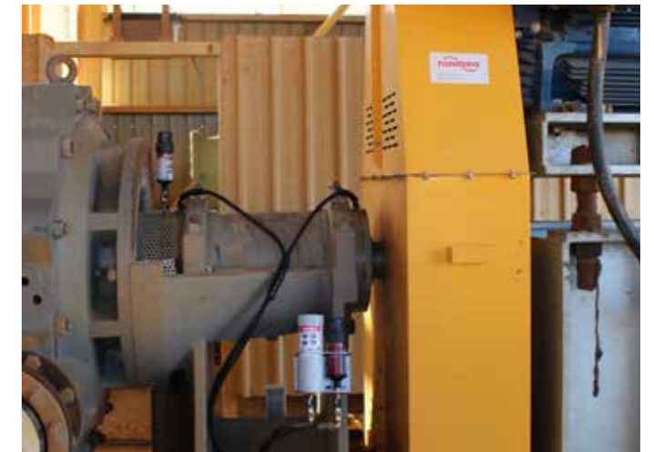
Application Horizontal slurry pump labyrinth seals and impeller mechanical seal Lubricator perma STAR VARIO L250 Installation kit K230C & direct mount
