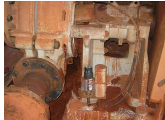
Application Horizontal slurry pump labyrinth seals Lubricator perma STAR VARIO L250 Installation kit K265C
