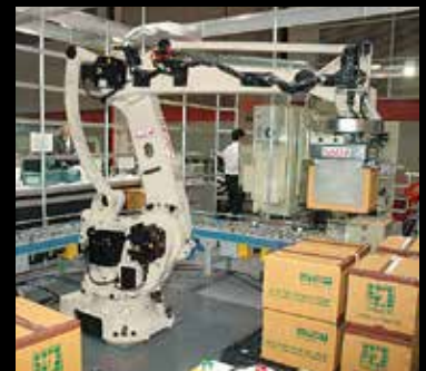
Palletising Robot "LP130/180" Enable high-speed/high-precision palletisation of cardboard boxes, bags, bottles, and metal products.
