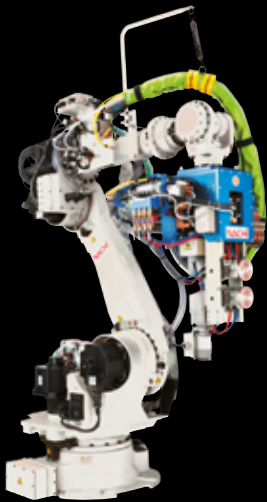
High-speed seam welding robots
