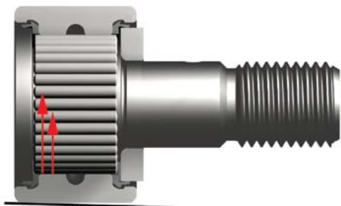
Cylindrical OD: Misalignment can cause corner loading
